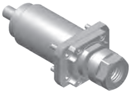
CCB721000 Drilling/milling unit RATIO 1 : 1 RPM(MAX) 6000 TOOL CLAMPING ER20A
